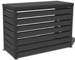
Horizontal Blades Blade Centre Spacing: 89mm Clear Gap: 24mm Blade Angle: 10°
