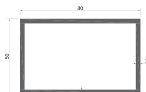
GM-NEWZ-80x50x3 GM-NEWZ-06 Hole Weight: 2.33kg/m
