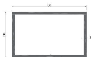
GM-NEWZ-80x50x3 GM-NEWZ-06 Hole Weight: 2.12kg/m
