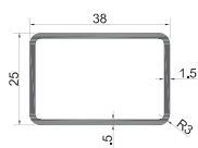
GM-NEWZ-38x25x1.5R Ø20mm Round Hole Weight: 0.523kg/m
