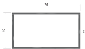
GM-NEWZ-75x40x2 GM-NEWZ-06 Hole Weight: 1.265kg/m
