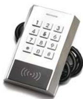
XKI-EM Secure Access Control Keypad Voltage Range: 12-28V Card Type: 13.56MHz Mifare Card Overall Size: 115x75x22mm Waterproof Rating: IP66
