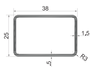
GM-NEWZ-38x25x1.5R Ø20mm Round Hole Weight: 0.523kg/m
