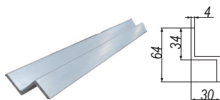
FG02A Aluminium Z-shape Track Material: Aluminium Weight: 1.1kg/m
