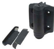
SHG-90C Self-closing Hinge with Safety Cap Max Holding weight: 28kg Fixing Holes: 4 Gaps: 9mm-28mm
