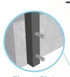
Flange Plate Use a Flange Plate when setting up posts
